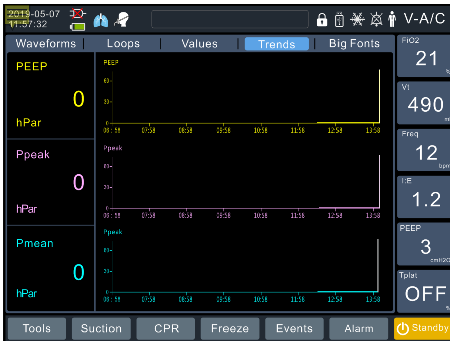
Fig. 22 Trend diagram interface
