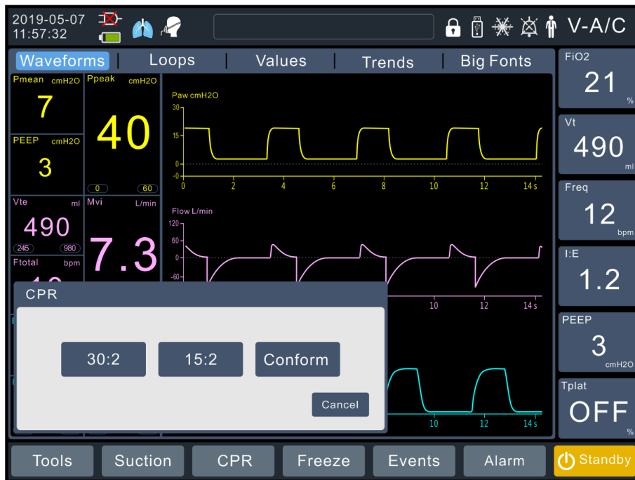
Fig. 26 CPR (select operation mode)
