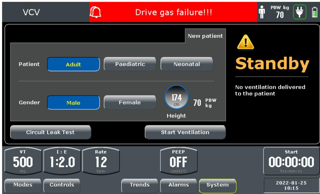
When the anesthetic workstation is on and not in use for a short time, it enters standby mode to save energy and prolong its life span.
